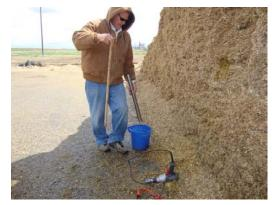
The most accurate measurements of packing density will come from corings taken within the top few feet of the silage pile. Samples taken lower are affected by compaction.
