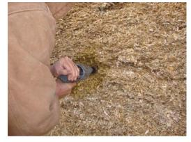
The coring drill is a standard size so by knowing the depth of the hole and weight of the silage removed from the hole, density can be calculated using a spreadsheet
